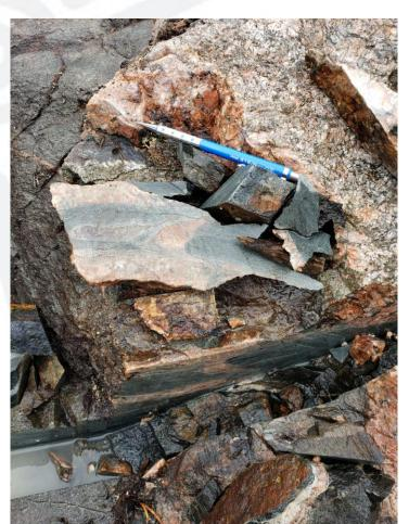
Figure 1. QFP dike with 0.5 to 1% pyrite mineralization along the newly cleared road.
