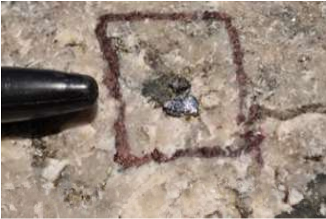
Photo of metallic silver molybdenite crystals in pegmatite outcrop on NMX East lithium property. Black Sharpie cap tip for scale.
