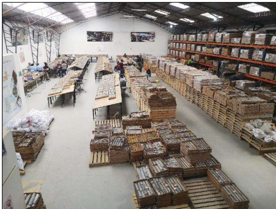
Figure 22: Warintza Project, Central Core Shed Facilities in Quito, Ecuador Source: GSI (2021)
