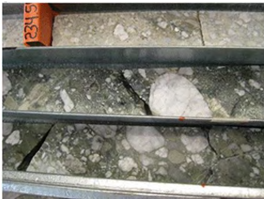
Figure 7.6. Photo of the basal quartz pebble conglomerate of the Amagá from drill hole MJ-6 (Maria Jo) at 234 meters (Source: Behre Dolbear, 2013)
