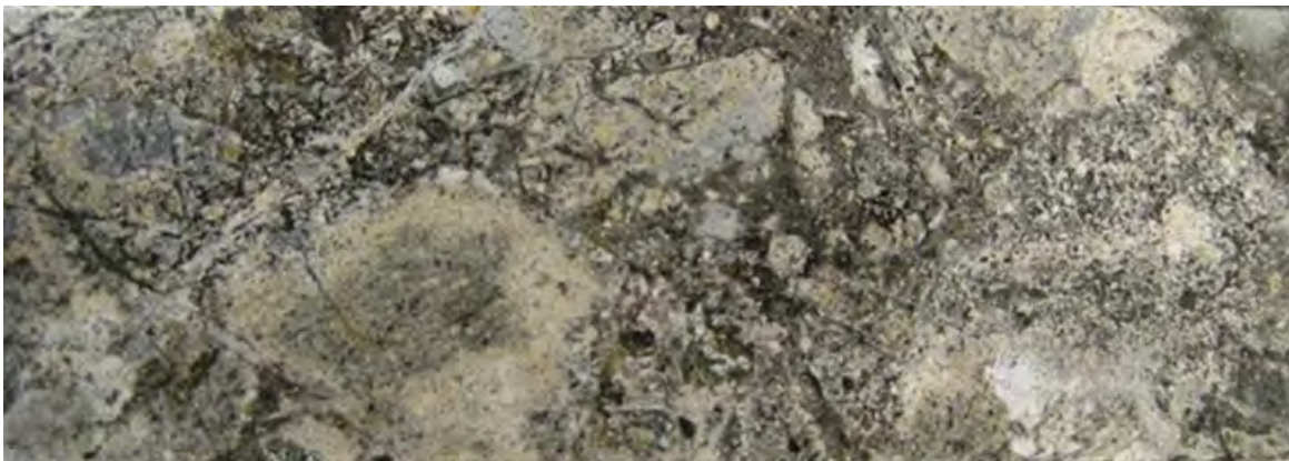
Figure 7.17. Diorite breccia with alteration halos on fragments from hole CV98 at 292 meters (assay interval contains 0.268 grams gold per tonne and 0.120% copper) (Source: Behre Dolbear, 2013)
