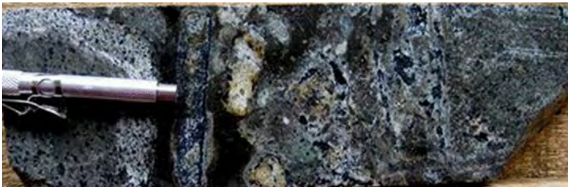
Figure 7.13. Intrusive breccia with magnetite-rich fragments, magnetite-rich matrix from drill hole CV038 at 208 meters (assay interval contains 0.3 grams of gold per tonne and 0.23% copper) (Source: Behre Dolbear, 2011)
